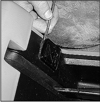
Remove power mirror controller by prying out
