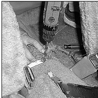
Drill mounting bracket holes out to 3/8"
