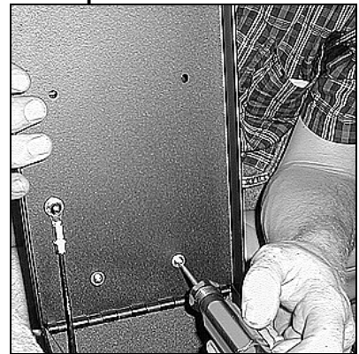
Using (2)#8x5/8", (3)#8x1" screws and (5) washers, screw lid cushion to Tuffy box.
