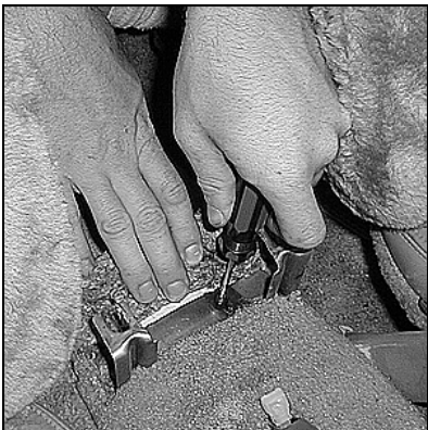
Remove rear mounting bracket from floor
