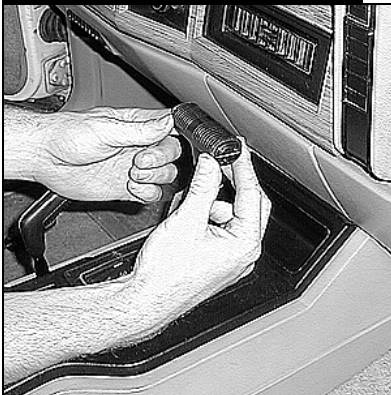
Remove shift lever handle by pulling straight up
