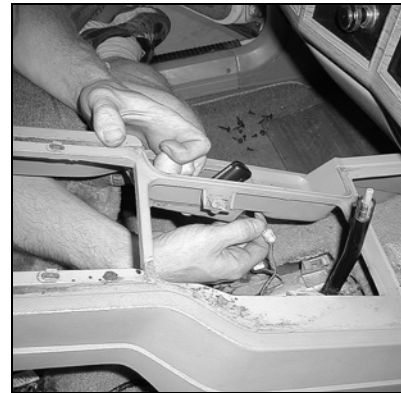
Remove console being careful to disconnect bulbs from shift bezels
