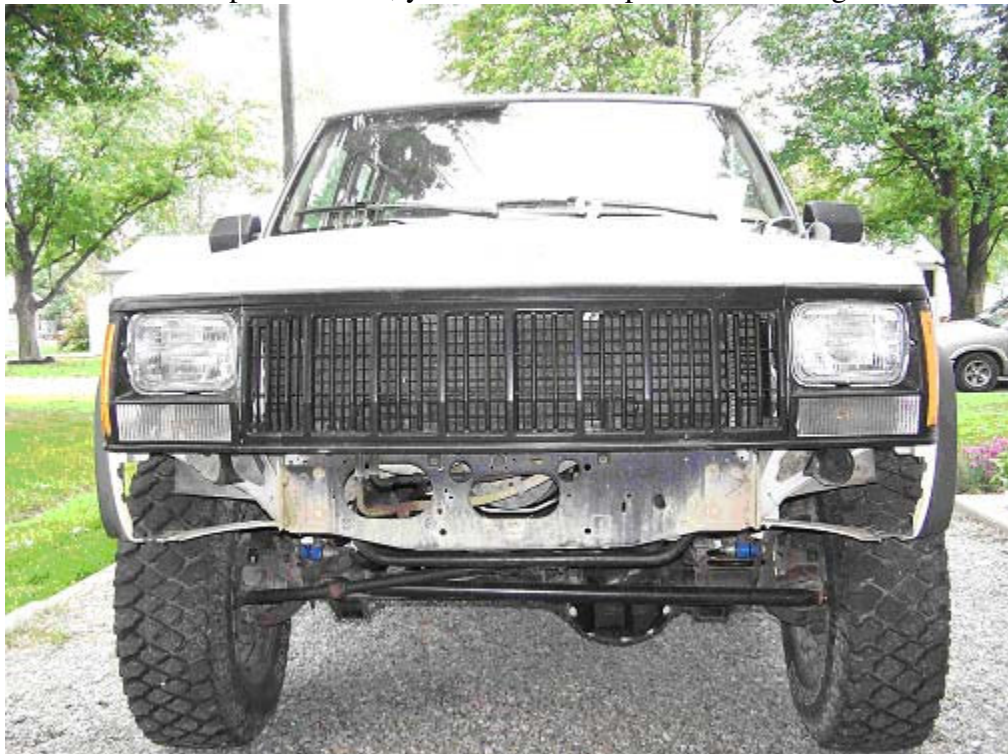
With the bumper removed, you should end up with something like this:
