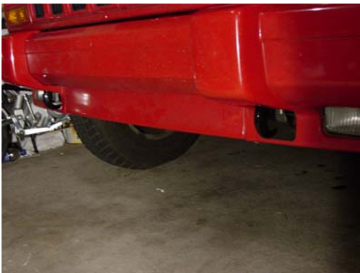
And here's the finished install with hooks and all. I used a box end wrench to hold the head of the bolt on the hooks, and a ratchet and deep-well socket to get the nuts on the bottom.
